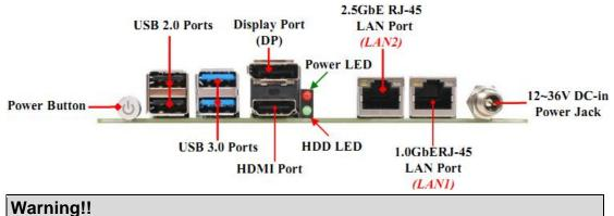
The board has a 12~36V DC-in power connector (**DCIN2**) in I/O back panel and an internal 12~36V power connector (**DCIN3**). User can only connect one type of compatible power supply to one of them to power the system.
