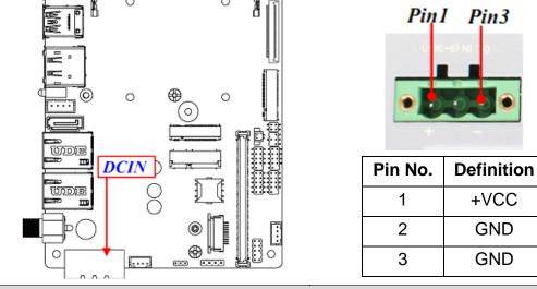
*Warning:* Find Pin-1 position before connecting power cable to this 3-pin power connector. *WRONG INSTALLATION DIRECTION WILL DAMAGE THE BOARD!!*
