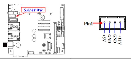
**Warning:** Make sure that Pin-1 of ompatible SATA Power out connector is inserted into corresponding Pin-1 of **SATAPWR** connector to avoid possible damage to the board and hard disk driver!
