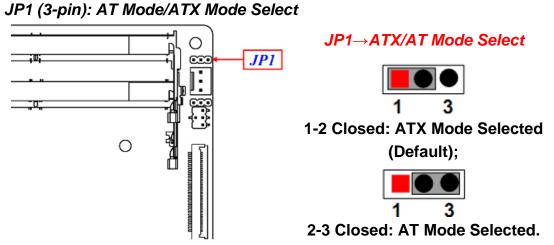
**\*ATX Mode Selected**: Press power button to power on after power input ready;
